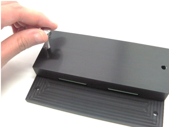
Figure 4. Setting up of the MED Duet Connector. Just putting the Top Unit on the Bottom Unit and fixing with the Fixing Screws.
