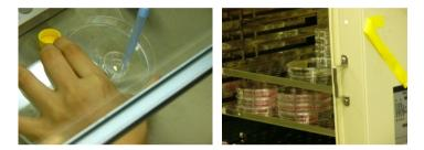
Figure 2. Rinse the MED Probe with PBS (left). Store the MED Probe filled with Laminin-511 in a sterilized dish and incubate it for up to 1 hr (right).
