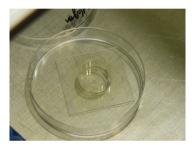
Figure 2. The MED Probe after completion of the coating. The electrodes should maintain moisture.
