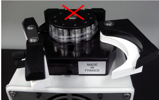
Figure 32. Bad examples for the tubes installed.
