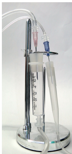
Figure 36. Inlet and Outlet drippers stranded at the dripper stand (left), and how they work to remove noises (right).
