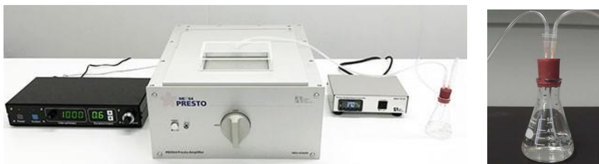
Figure 3-1. Experimental environment for the MED64 Presto system (left). Bubble the gas through a beaker containing distilled water to maintain a humidified environment (right).
