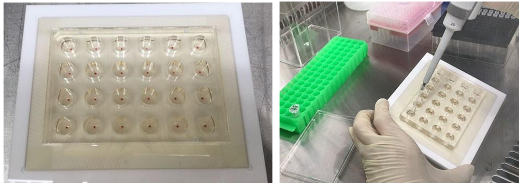
Figure 2-1. MEA Plate24-eco loaded on the CellDroplet24. Location of electrodes are marked with red color (left). Dispensing the fibronectin solution onto the recording electrodes in a well.
