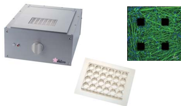
FIGURE 1: The MED64 Presto high throughput MEA (left) and Axol stem cell-derived sensory neurons plated onto MEA electrodes (right).
