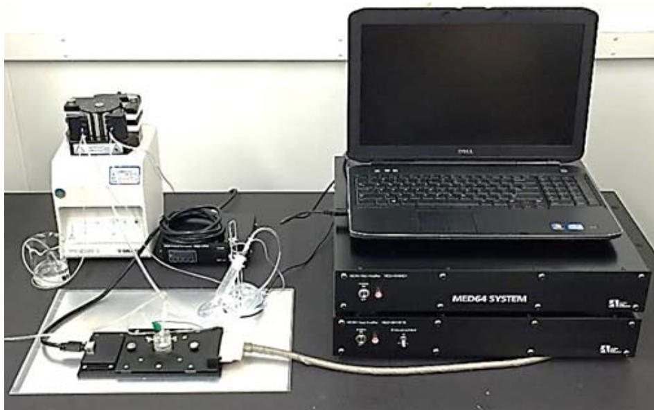
Figure 6. MED64-Basic System with perfusion system installed on a lab bench.
