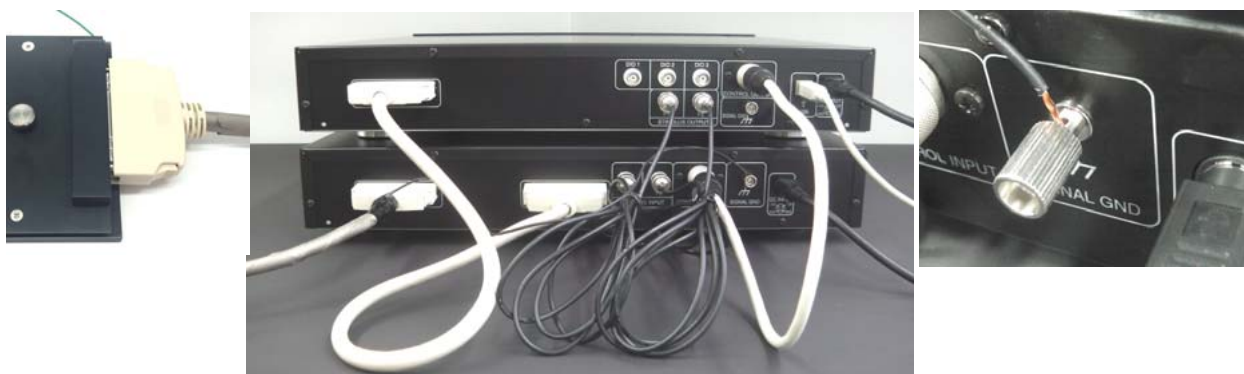
Figure 10. Connection between the MED ThermoConnector and amplifiers. Connection for the Connector cable (left), Connection for amplifiers (middle) and grounding for the MED Connector cable (right).
