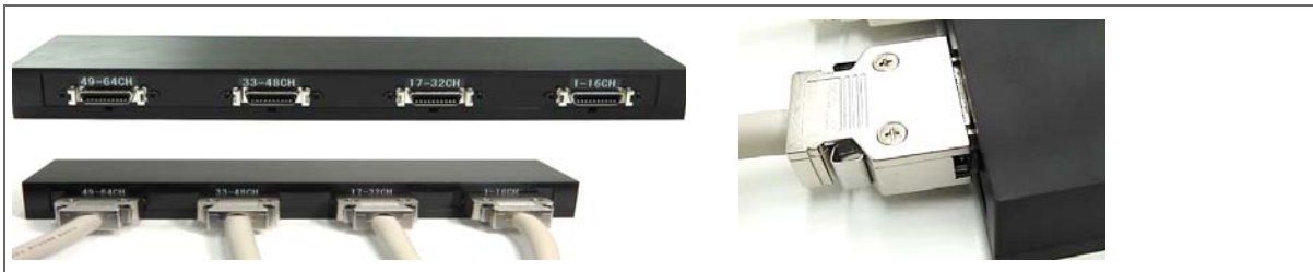
Figure 4. Connecting the MED Connector cables (20 pins) to the MED Multi-well Connector.
