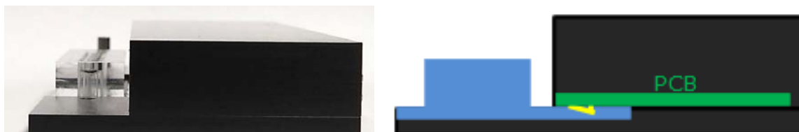
Figure 15. MED Multi-well Probe. View from side (left) and its structural scheme (right).
