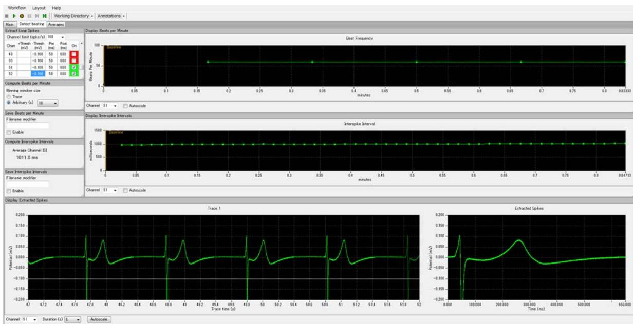
Figure 4-3.34. Analysis performed with the "Beat\_frequency\_analysis" workflow template. Beats (long spikes) are counted by every 10 seconds and displayed on the [Display Beats per Minute] module. (top-graph) Interspike intervals are measured and graphed in the [Display Interspike Intervals] module (center graph). The bottom graphs show long spikes that are extracted over time (high-lighted with light-green) (left) and each extracted long spike (right).
