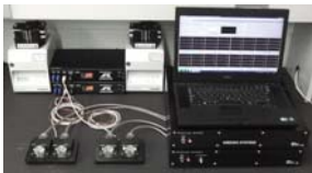
MED64-Quad II platform with perfusion accessories (left) and MED Probe 16, MEA (right).
