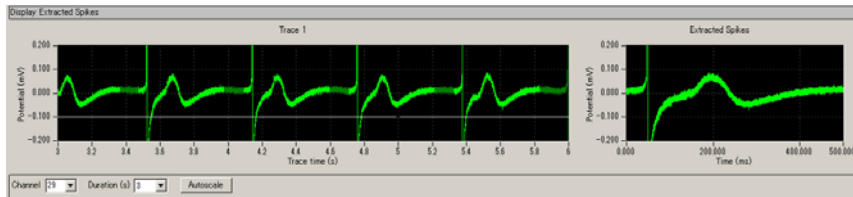
Fig. 4-3.14. Long spikes are extracted (high-lighted with light green color).
