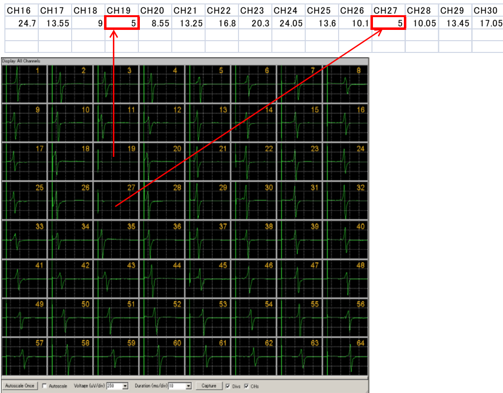
Fig.4-5.14. The values for stimulation channels (19 and 27) were changed to the pre-stimulation time (5 msec). (top).
