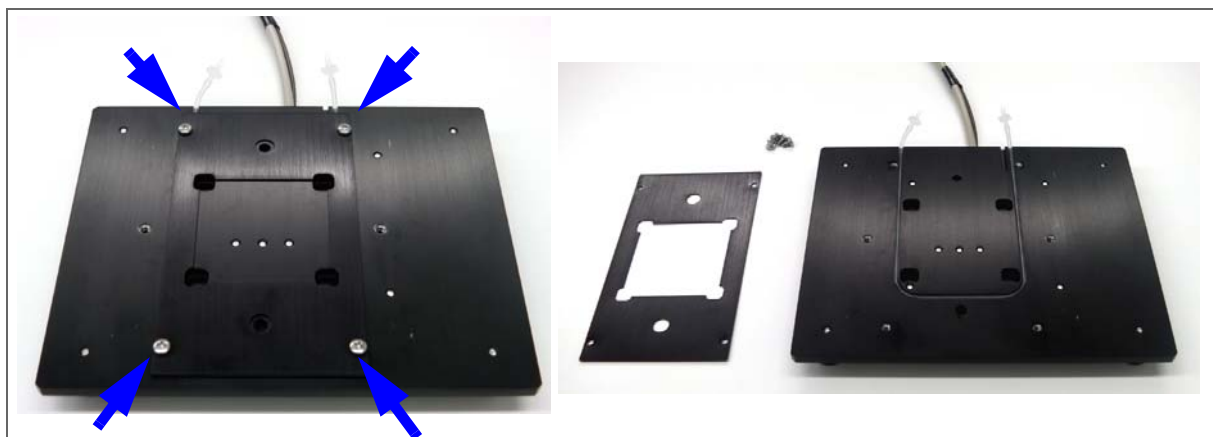
Figure 16. Removing the aluminum plate from the heater base.
