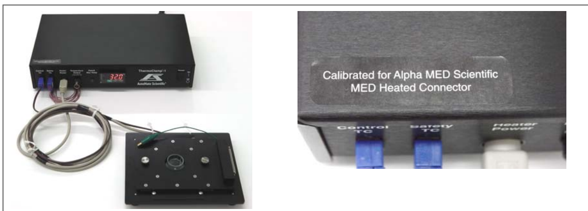
Figure 4. The MED Heated Connector connected to the ThermoClamp™-1 (left), and the label on the ThermoClamp™-1. This ThermoClamp™-1 can be used ONLY with the MED Heated Connector.
