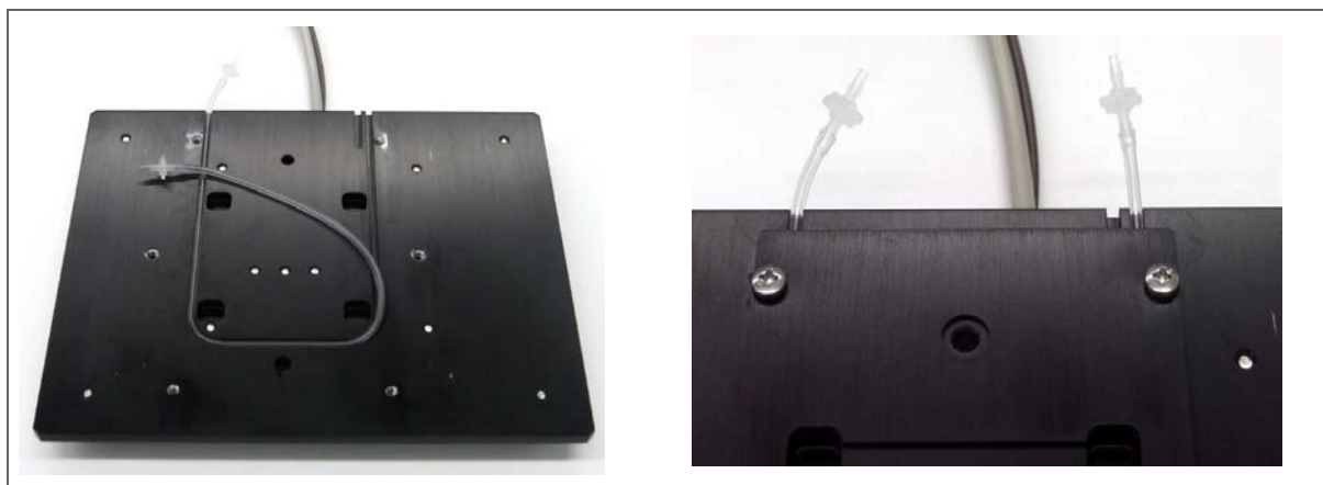
Figure 17. Removing the tube (left) and the aluminum plate returned (right).
