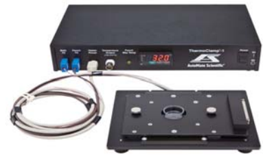
Fig. 4. The MED Heated Connector connected to the ThermoClamp™-1.
