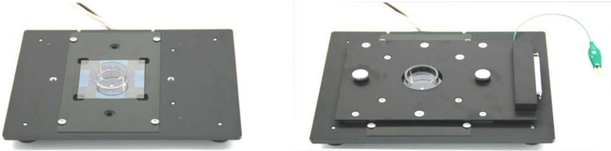
Fig. 8. Installing the MED Probe onto the Heated Connector.
