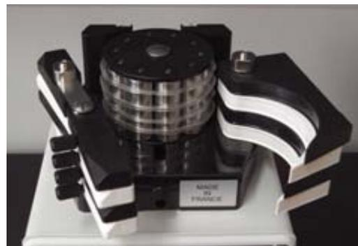
4. Make sure that all tubes are installed horizontally so that they sit under each compression cam.
