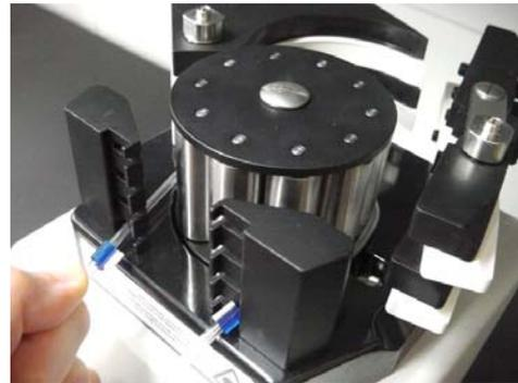
2. Install the tube to the rollers.
