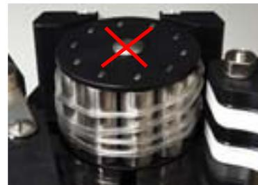
7. Bad example: tubes are not installed horizontally.
