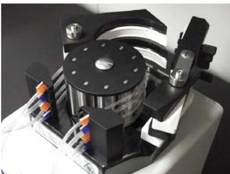
3. Outlet(orange)/Inlet(blue) tubes installed to the Minipuls 3.
