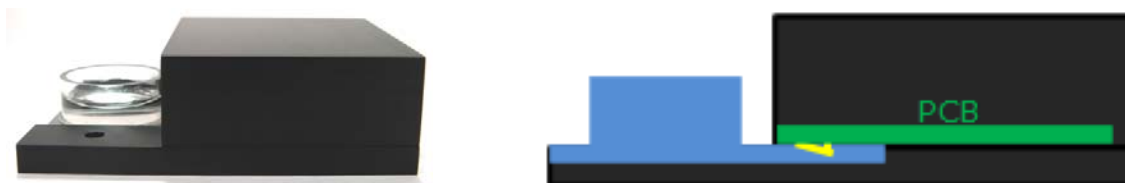
Figure 13. MED Mini Connector where the MED Probe 16 is loaded (left). View from side (left) and its structural scheme (right).
