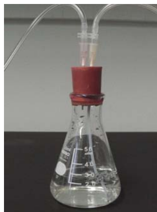
Figure 2. Equipment for microenvironmental control. A. Complete experimental set up with the MED Heated Connector/ThermoClamp™-1 controller and MED Connector Cover. B. Bubble the gas through a beaker containing distilled water to maintain a humidified environment.
