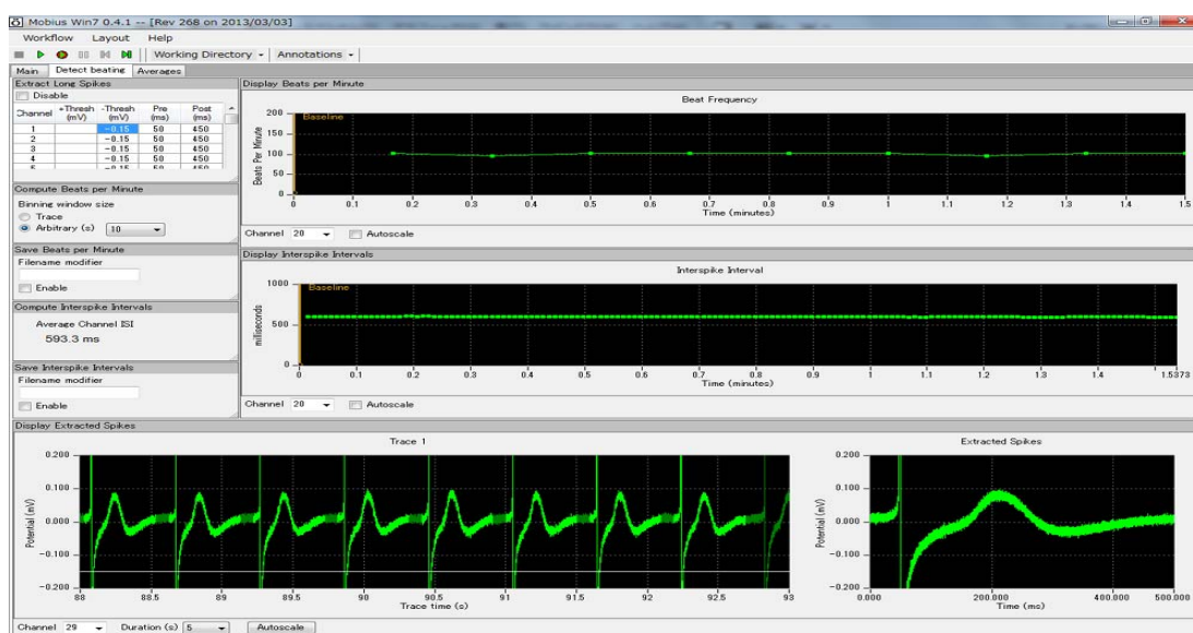
Figure 3. Screen shot of Mobius QT's built-in workflow for beat frequency analysis. Cardiac signals that surpass user-determined thresholds are extracted. Beat frequencies and ISI can be saved as ASCII files. Beat frequencies and interspike intervals (ISI) are computed and graphed.
