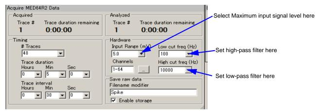
Setting of acquisition-bandwidth and Gain on the Mobius' [Acquire MED64R2 Data] module. The acquisition-bandwidth is now set for 100 Hz -10 kHz and the Gain is x100.
