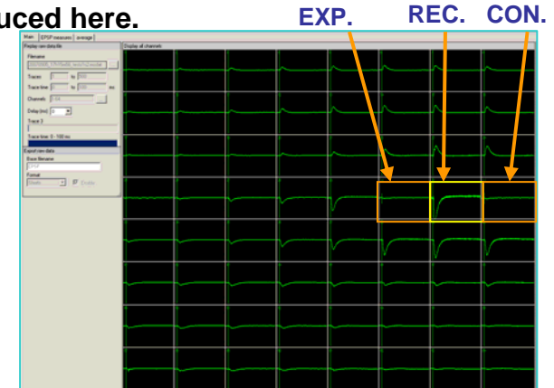
Figure. L-2: Look for the stimulation points while changing the stimulation points. In this example, channels are selected as follows: (EXP: Ch30, CONTROL:Ch32, On-line analysis Ch.31)
